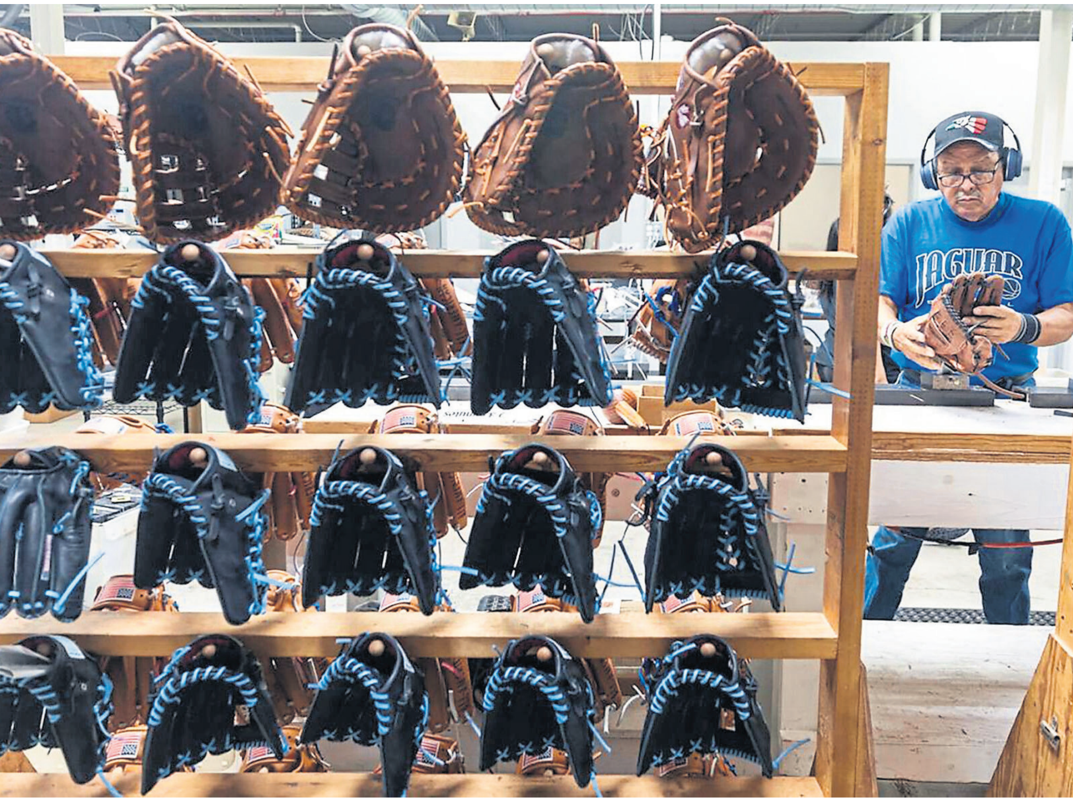
Ricardo Carranza uses a heated metal insert to shape the inside of the glove.
