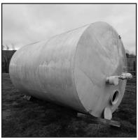
cleaned up etc before using. We messed up the sight tube ports when we moved it home so that will need reworked. The main port will be fine if the threads are brushed out etc. We turned the valve off of it fine but it's been sitting for 3 years now.
